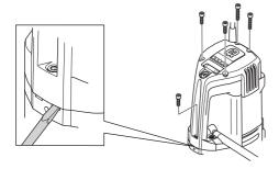
2 Lift the brush retainer spring to one side (1).
