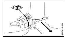
When making the felling notch, use the gunning sight on the shroud and housing to check the desired direction of fall:
