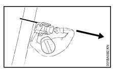
Position the chain saw in such a way that your body is clear of the cutting attachment whenever the engine is running. Stand to the left of cut while bucking.
