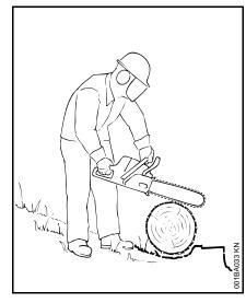
Bucking is cutting a log into sections.
