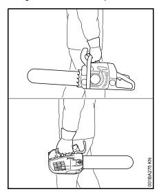
By hand: When transporting your chain saw by hand, the engine must be shut off and the chain saw must be in the proper position, i.e., grip the top handle and place the muffler away from the body; the chain guard (scabbard) should be over the saw chain and guide bar, which should point backwards, away from the direction in which you are walking.
