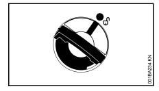
To do this with this STIHL cap, raise the grip on the top of the cap until it is upright at a 90° angle. Insert the cap in the fuel tank with the positioning mark on the grip of the cap and the "open" mark on the fuel tank opening lining up. Using the grip, press the cap down firmly while turning it clockwise as far as it will go
