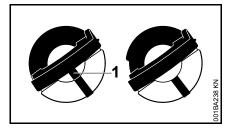
Left: Bottom of cap in closed position - inner mark (1) in line with outer mark.
