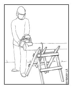
When cutting small logs, place log through "V"-shaped supports on top of a sawhorse. Never permit another person to hold the log. Never hold the log with your leg or foot.
