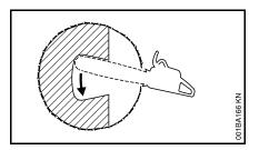
Enlarge the plunge cut as shown in the illustration.
