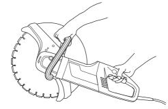
• Press in the power switch lock with your right-hand thumb and press in the power switch.
