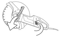
In order for the machine to always be cooled sufficiently the cooling air openings must be kept clear and clean. Blow down the machine regularly with compressed air.
