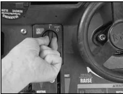
(A) Place Engine Master Switch in the OFF position.
