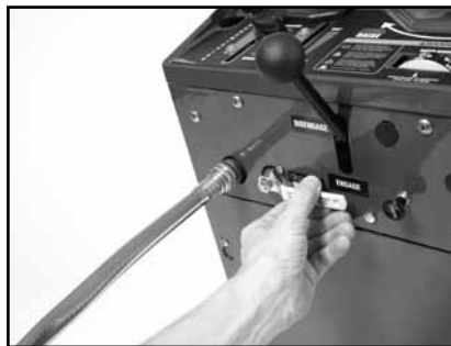
(H) For Wet Cutting, open Cooling Supply Valve. Verify proper cooling flow and adjust the water flow on the Blade to a desired amount.
