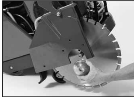
(E) Install the Outer Flange. Verify the drive pin is seated; it must project through the hole in the blade and into the flange.
