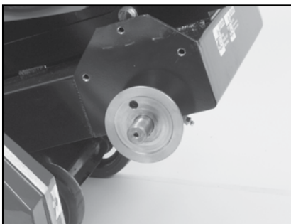
(E) Clean and lubricate the Blade Shaft.
