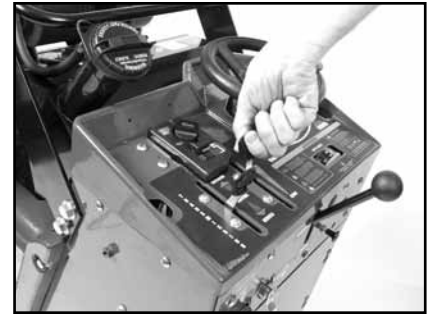
(F) Push Engine Throttle Handle up half-way.
