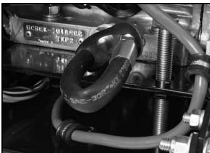
(A) Verify the Oil Drain Cap is installed onto the Oil Drain Line and is tight. Refer to Engine Manual for details.
