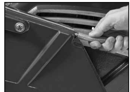
(I) Install the Cooling Transfer Hose to the Blade Guard.
