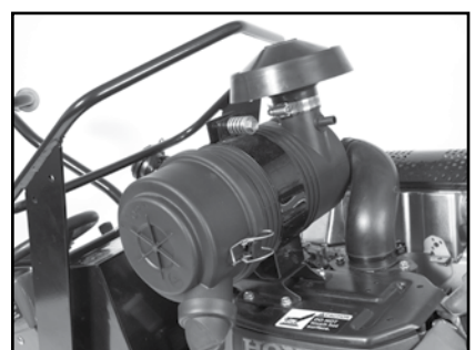
(C) Clean engine Air Filter weekly and replace monthly. Refer to Engine Manual for details.
