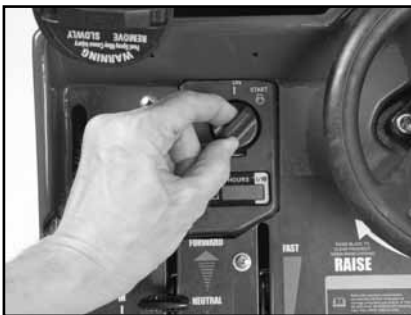
(G) Start engine by rotating Ignition Switch to the right.
