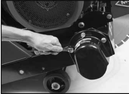
(J) Install the Blade Shaft Cover.
