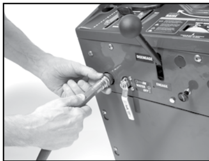
(B) Attach the cooling supply hose to the Cooling Inlet, if wet cutting.
