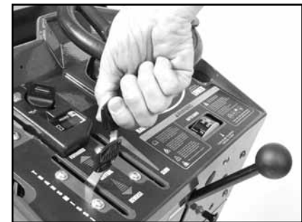
(I) Move the throttle all the way for- ward to "Fast" position.
