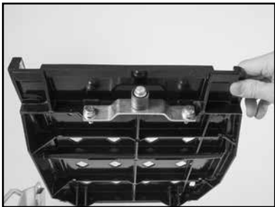
(D) Verify the Roller Wheel Assembly is tight and in good condition.
