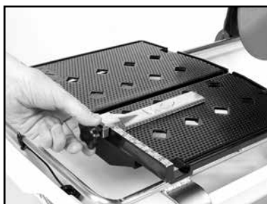
(B) Place the Adjustable Cutting Guide onto the Movable Cutting Table Ruler/Stop and tighten the retaining thumbscrew
