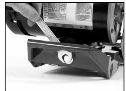
(I) Loosen the Motor Adjustment Strap
