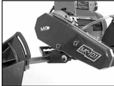
(B) Remove the Cutting Head from the rear pivot hole
