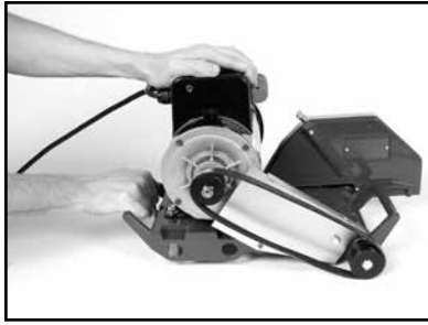
(J) Push the motor toward the front of the Cutting Head to loosen the Micro-V Belt
