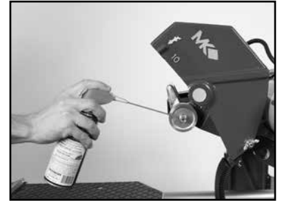
(C) Lubricate the Inner Flange
