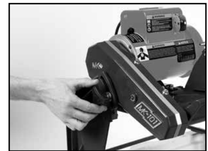
(C) Ensure the Adjusting Knob is tight
