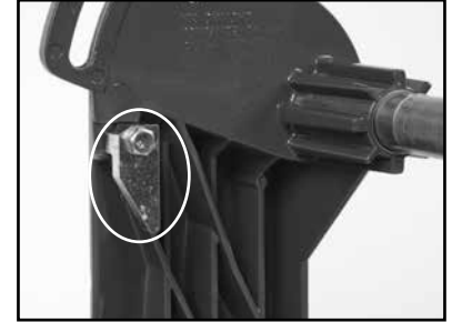
(C) Move Cutting Head Stop to down position
