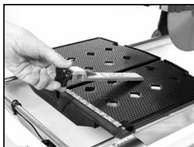
(A) Loosen Adjustable Cutting Guide retaining thumbscrew and place it over the Movable Cutting Table Ruler/Stop
