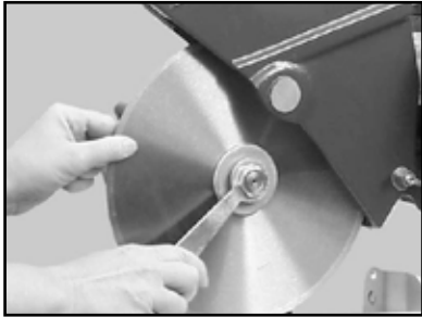
(A) Remove the Diamond Blade
