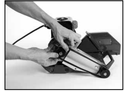
(L) Install the new Micro-V Belt (MK Diamond Part No. 158194)
