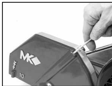
(H) Rod Cooling Channels and recheck flow
