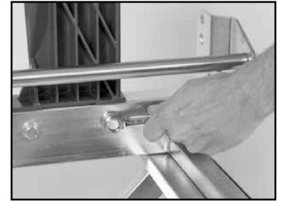
(C) Loosen the Retaining Bolts.
