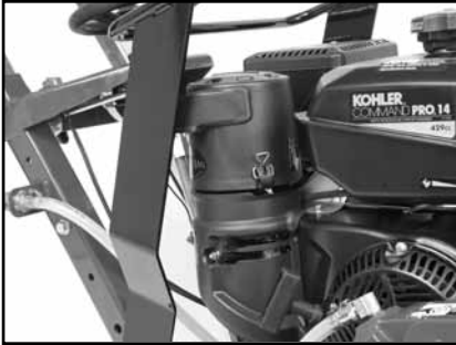
(D) Clean engine Air Filter weekly and replace monthly. Refer to Engine Manual for details.
