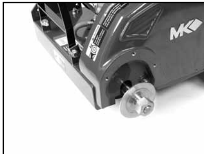
(G) Clean and lubricate the Blade Retaining Bolt.
