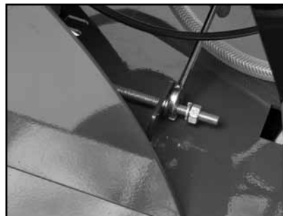
(G) Loosen Jam Nut on Engine Tension Arm.
