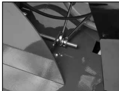
(H) Loosen the Engine Tension Arm adjusting nut. Push the Engine forward to loosen the belt.
