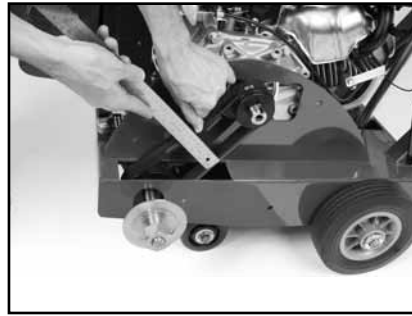
(N) Check belt for proper tension (Proper tension is approximately 1/8-inch deflection of the belt).
