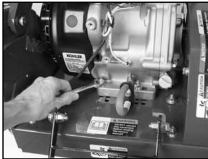
(E) Locate the four upper Engine Mounting Nuts on both ends of the motor and loosen.
