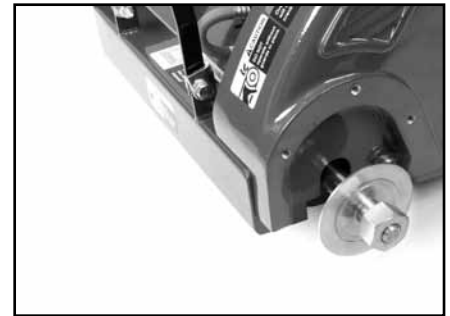
(F) Remove the Blade Shaft Cover Retaining Bolts and the Blade Shaft Cover.
