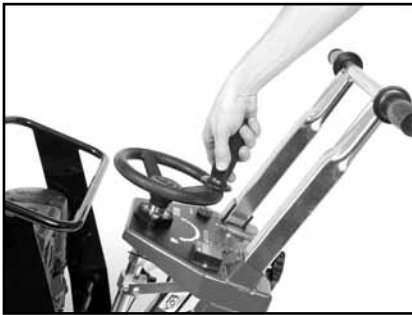
(A) Use the Depth Control Wheel to raise the blade clear of the floor.
