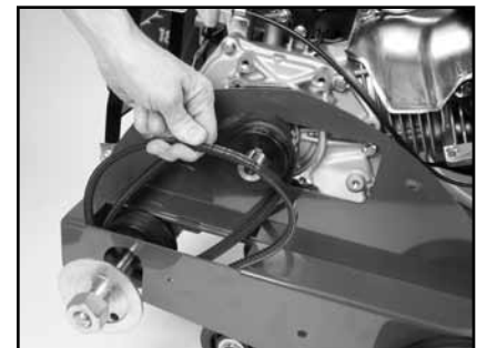
(I) Remove the old belts from the Engine and Blade Shaft Pulleys.
