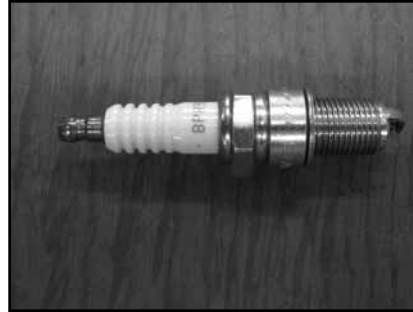
(E) Clean Spark Plug Weekly and readjust Spark Plug monthly. Refer to Engine Manual for details.
