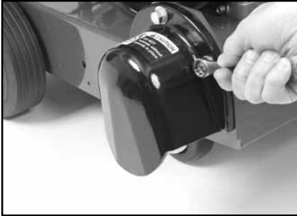
(J) Install the Blade Shaft Cover.
