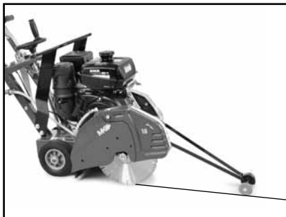
(D) Layout and mark the area to be cut using a chalk-line. Align Pointer and Blade to chalk-line.
