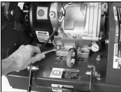
(P) Tighten the Engine Mounting Bolts.
