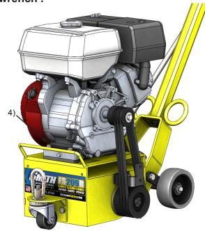
5. Slide the engine back enough to remove and replace the belts as necessary.
